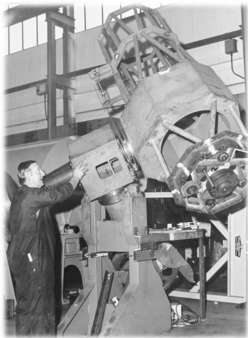
Figure 10 The 24" Thornton reflector being built in the William Boulton workshops, with Chief Fitter Mr. Davenport.
