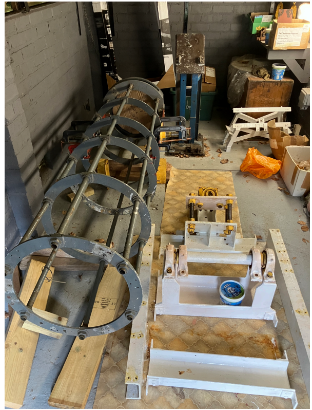
Figure 5 Inside the Hindle enclosure: the telescope truss on the left and base of the mount in the centre. The pillar of the 10" Meade is still in place at the back.
