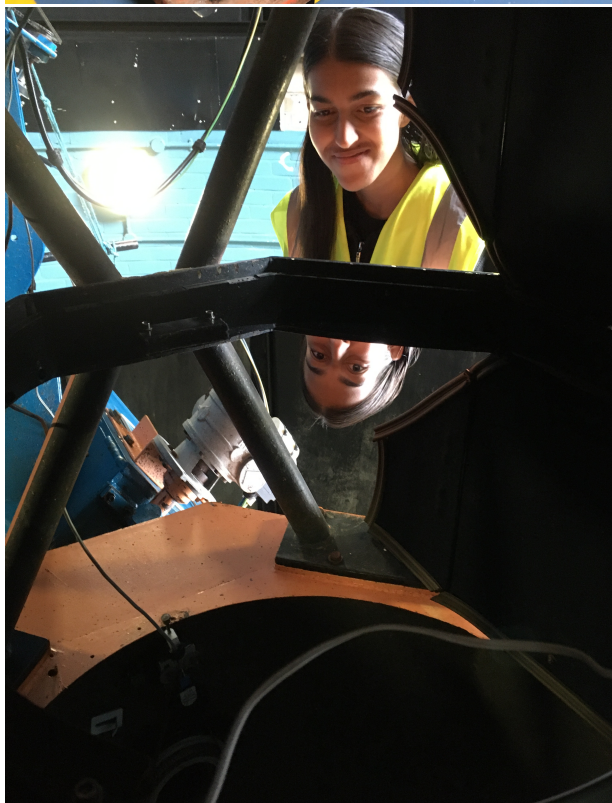
Figure 8 Natascha Dury inspects the 24" mirror being reinstalled after having been recoated by Galvoptics.
