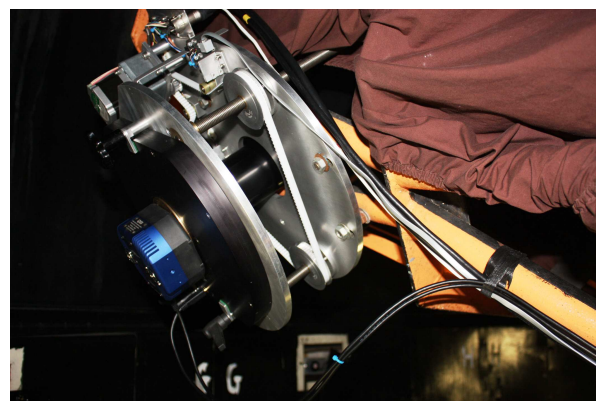
Figure 5 QSI camera and filterwheel on the focus platform at the 24" reflector. Credit: StJohn Robinson.
