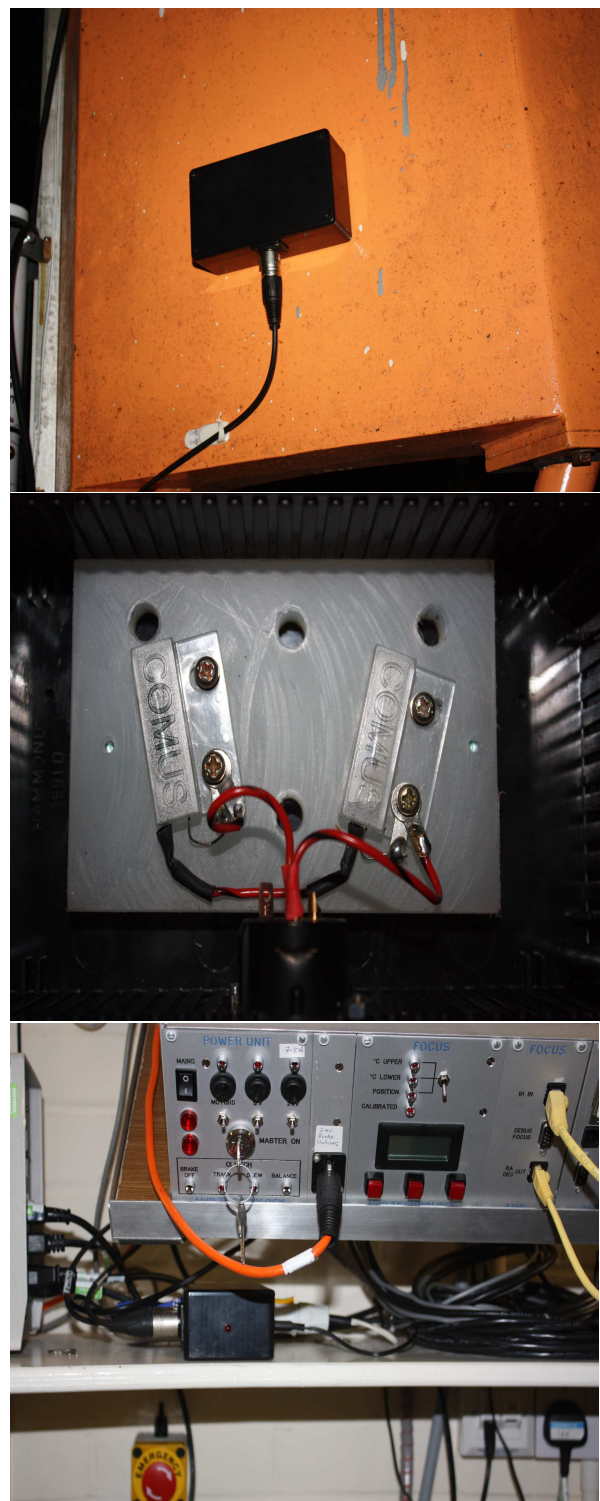
Figure 7 Mercury tilt switches installed on the side of the 24" truss (top), seen inside the box (middle), with an indicator unit in the control room (bottom, below the AWR electronics rack). Credit: StJohn Robinson.
