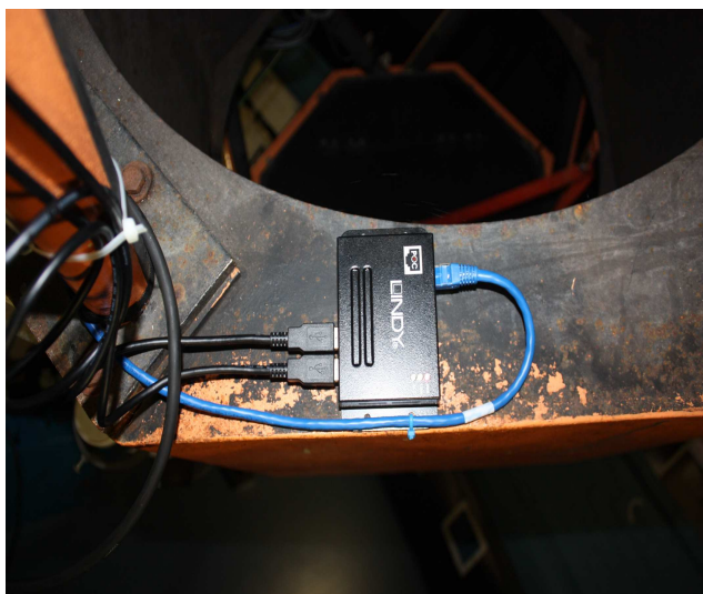
Figure 6 USB-over-Ethernet hub replacing unreliable self-powered USB cables. Credit: StJohn Robinson.
