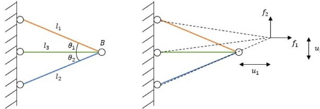
Figure 1: A simple truss structure before and after the application of forces at point  $B$ .
