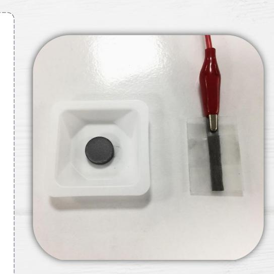
Composition of a pellet optimised at 40wt% of NaX zeolite Near-Nernstian response of 55.1±3.7 mV/decade
