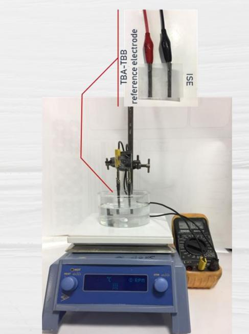
Mulitmeter measurements provide the near-Nernstian slope Solid contact reference electrode can be used instead of a classic one
