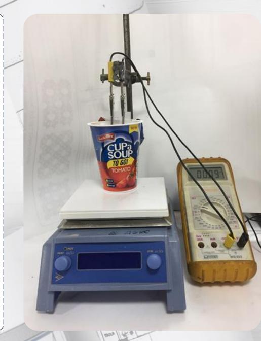
Real-life samples (bottled water and instant soups) have been tested Total amount of ions is detected
