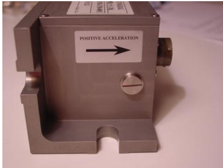
Figure C4 CMG-5U sensor showing positive acceleration direction
