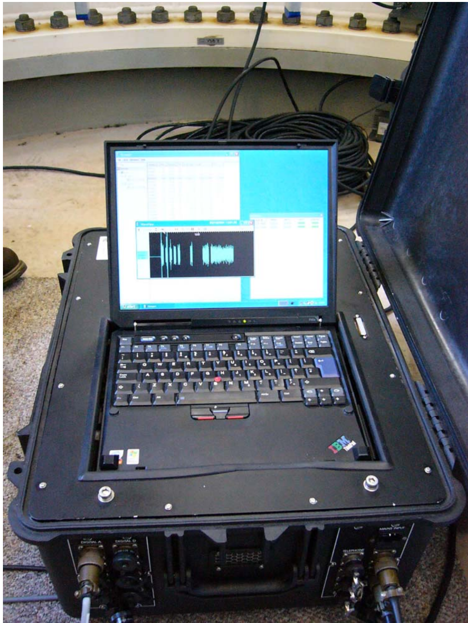
Figure C8 CMG-DM24S12AMS acquisition and monitoring system
