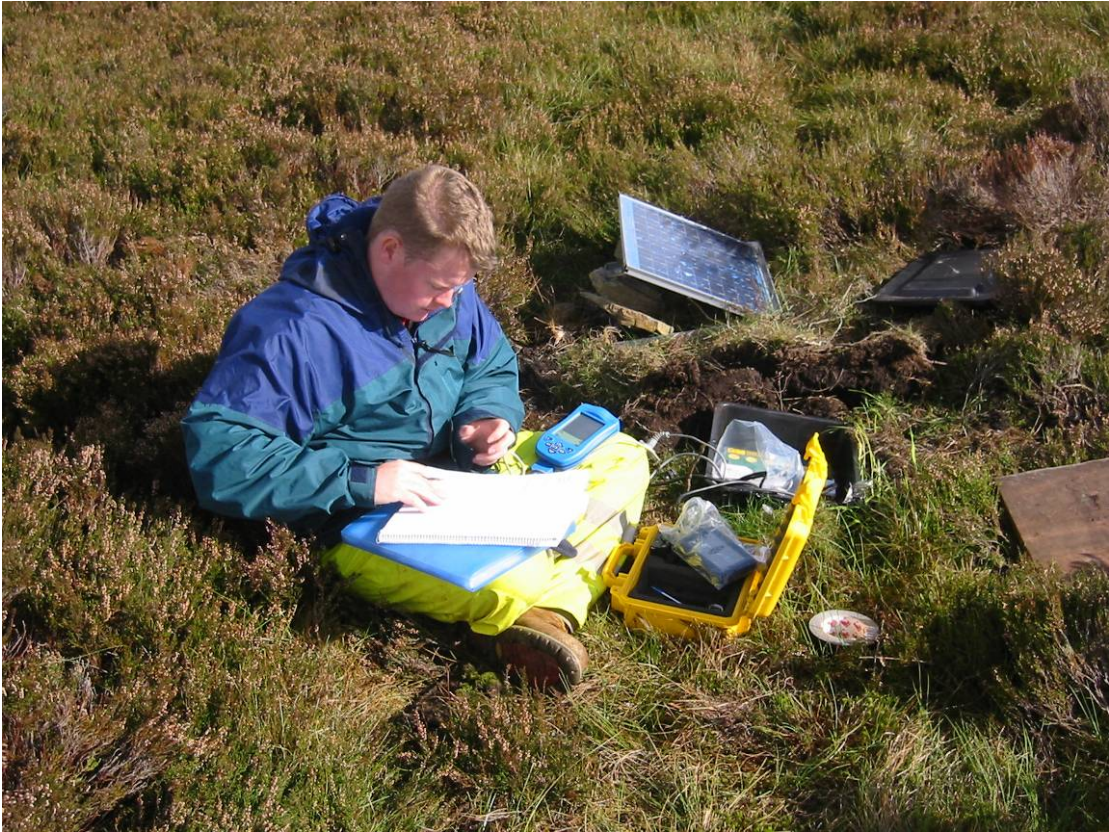
Figure A4 Servicing a CMG-6TD in the field
