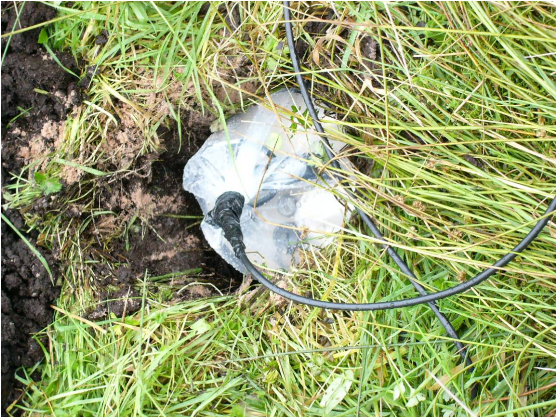
Figure C7 A CMG-5TD installed in the ground at Dun Law Windfarm.
